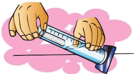
4. Tell students that you want to find out how much the water level changed. Subtract the initial water level from the final water level to find the volume of the rod.
